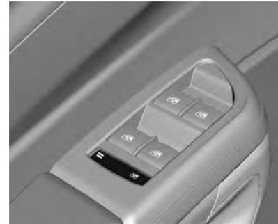
Pressione o interruptor
