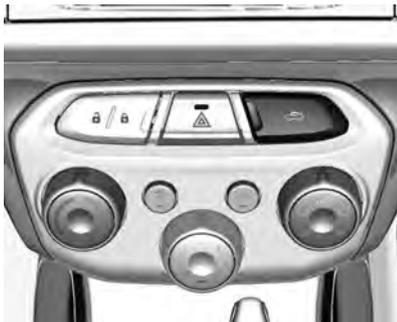
Para destravar e abrir a tampa do compartimento de carga, pressione o botão
