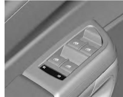
Pressione o interruptor
